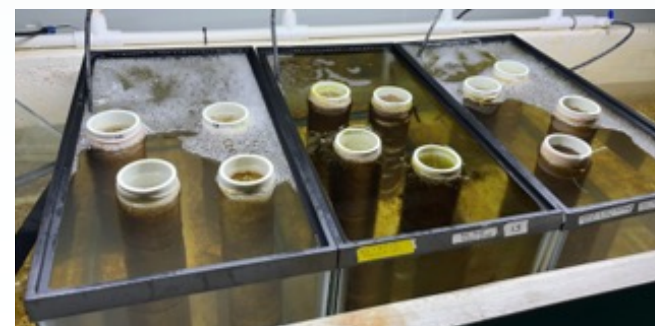
Figure 7 Post-experiment contamination (cloudy water, green coloring) resulting from increased nutrients and missed water changes. Picture by Carly Buchwald.
